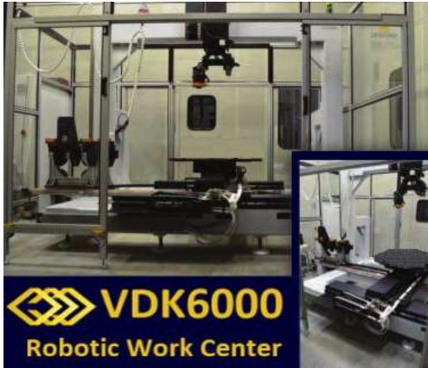
Six degree of freedom VDK6000 Robotic Center provides a unique, on the market, modular motion solution for advancing hybrid (additive and subtractive) manufacturing technology for creation and/or mending of complex metal parts.
